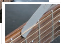
Checking a relief of the neck
