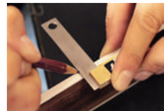
Marking for side position.
