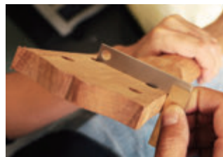
Checking flatness for installing machine heads
