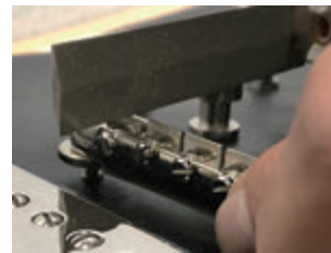
Good to make notches for strings on the metal saddles.
