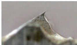
Enlarged CP files tooth. This tooth shape is the secret of why CP file works fine!
